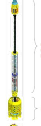
ULP & LUB TUB — Upper Lubricator Package & Lubricator Tubular
